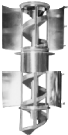
Enclosed transfer chute designed for through-floor installation
